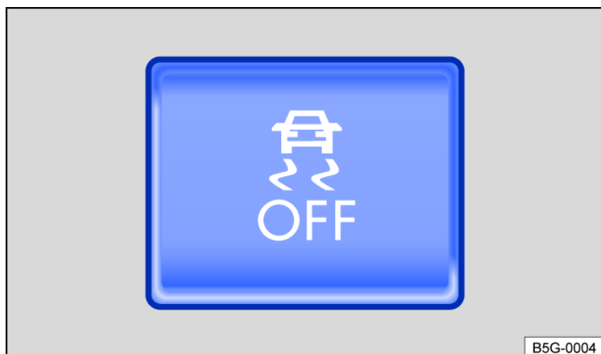
Fig. 121 Located on the center console: Button to manually switch ASR or ESC Sport on and off (depending on how your vehicle is equipped).
