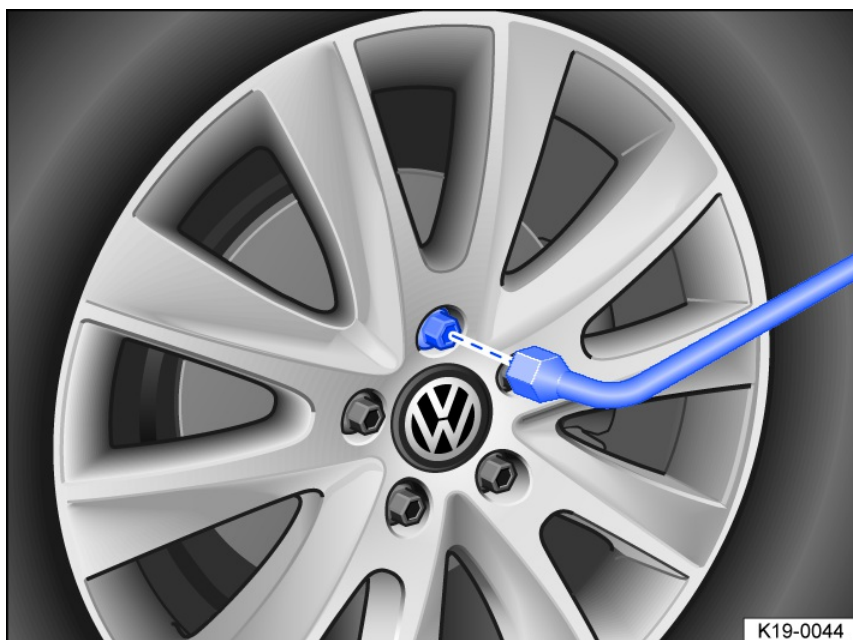
Fig. 213 Wheel change: removing wheel bolts with the lug wrench.
