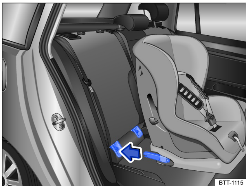
Fig. 42 General example: Installing a child restraint with attachment arms.
