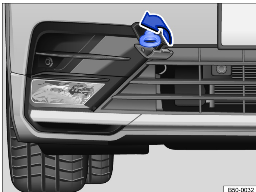
Fig. 186 In the right front bumper: Screw in towing eye.
