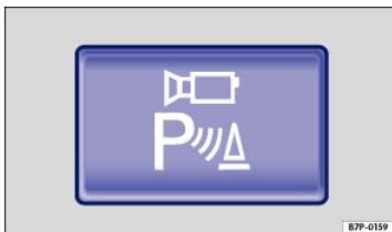
Fig. 142 In the lower center console: Button to switch Area View on.
