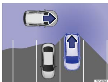
Fig. 140 Rear Traffic Alert: Monitored area around the vehicle that is backing out of a parking space.
