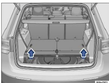
Fig. 192 In the luggage compartment for vehicles with seven seats: Pull straps to lift third row bench and access the compact spare wheel.
