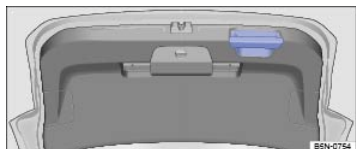
Fig. 63 Open trunk lid: Handle for closing the trunk lid.
