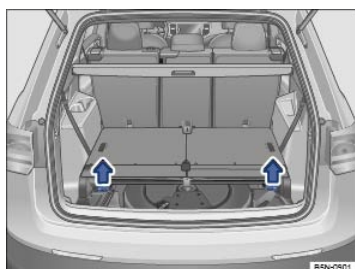
Fig. 153 In the luggage compartment for vehicles with seven seats: Pull straps to lift third row bench and access the subwoofer.
