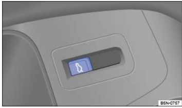
Fig. 55 In the driver door: Switch for the trunk lid (if equipped).
