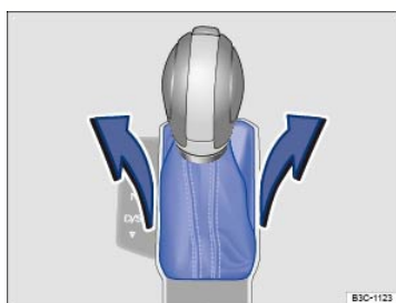
Fig. 118 Removing the selector gate cover.
