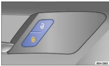
Fig. 54 In the driver and front passenger doors: Power locking switch.
