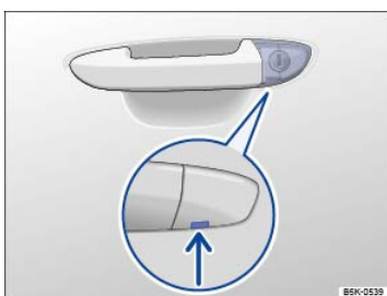
Fig. 56 Driver door: Concealed lock cylinder.
