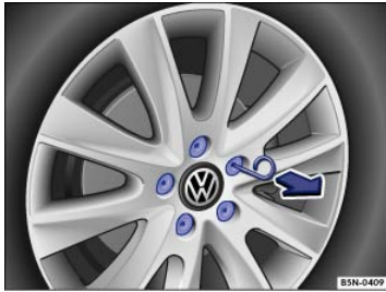
Fig. 196 Pulling cover caps off wheel bolts.
