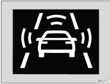
Fig. 131 In the instrument cluster display: Advance warning (symbol displayed in color on an instrument cluster with color display).
