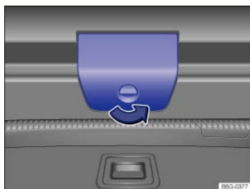
Fig. 68 Inside the luggage compartment: Cover for the trunk lid release.
