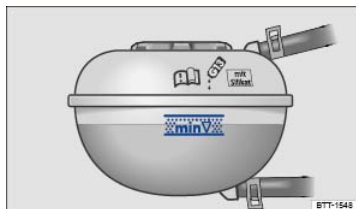
Fig. 186 Coolant expansion tank in the engine compartment.
