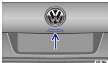
Fig. 62 In the trunk lid: Button to open the trunk lid.
