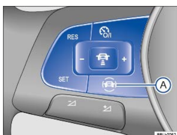
Fig. 18 On the multi-function steering wheel: Driver assistance systems button.
