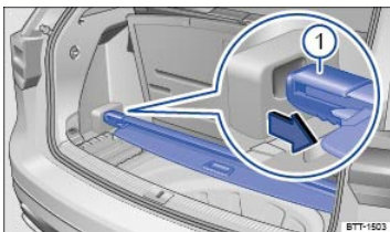
Fig. 158 Under the luggage compartment floor: Stowing the luggage compartment cover.
