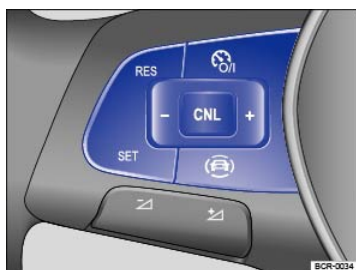
Fig. 126 Left-hand side of the multi-function steering wheel: Buttons for operating the cruise control.
