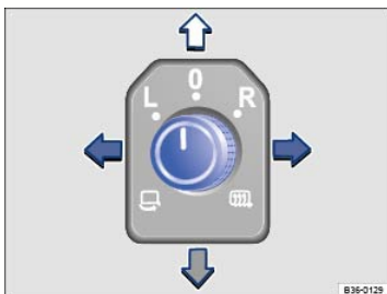
Fig. 101 In the driver door: Adjusting knob for the outside mirrors.
