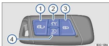
Fig. 113 Remote control vehicle key with remote start button.
