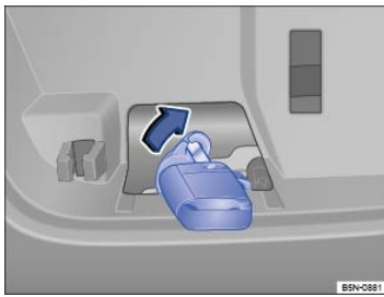
Fig. 69 Inside the luggage compartment, behind the cover: Opening the trunk lid.
