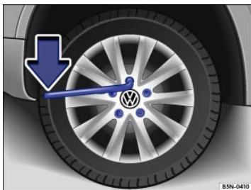
Fig. 197 Changing a wheel: Loosening the wheel bolts.
