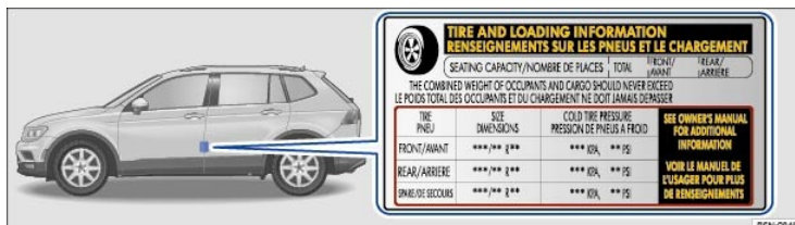
Fig. 190 On the driver door jamb: Location of the tire inflation pressure label.
