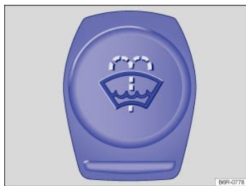
Fig. 183 In the engine compartment: Cap of the windshield washer fluid reservoir.
